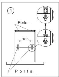
2.Move the retractable brackets into working position before installation. To do this, it is necessary to slightly loosen the screw holding them. After tightening the screw all the way, pull it out.
