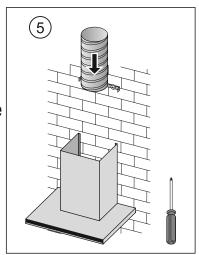
4.Install the chimney connection plate and fix it with the screws from the installation kit.
