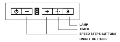
On/Off button: Touching this area will start working at the 2nd speed level when you turn on the product. Press this field to turn off the product while it is running.
