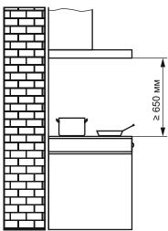
If there is a stove, gas boiler or column in the room, care should be taken to ensure that the hood receives the necessary air to avoid burning during operation. This also applies to rooms with closed windows and doors.
